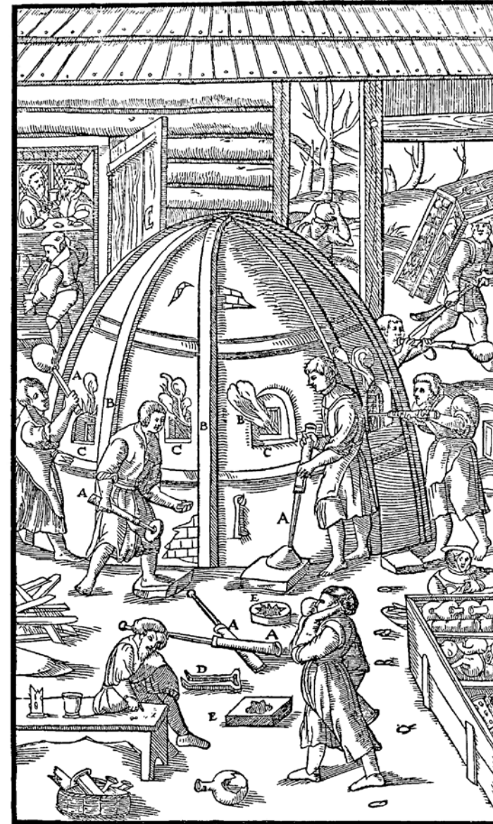
A—BLOW-PIPE. B—LITTLE WINDOW. C—MARBLE. D—FORCEPS. E—MOULDS BY MEANS OF WHICH THE SHAPES ARE PRODUCED.
